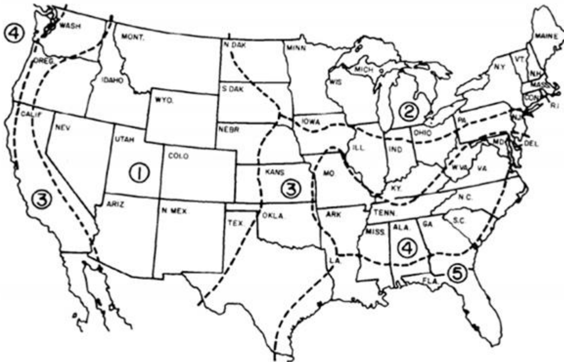
Figure 3-8 RUS Decay severity zones for wood poles (1= least severe, 5= most severe)
