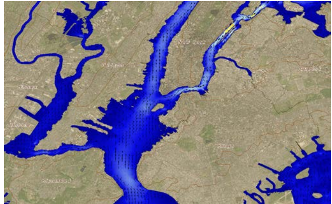
Figure 7: showing the Existing FEMA’s 2-D ADCIRC Coastal Model developed by Dewberry for New Jersey/New York
