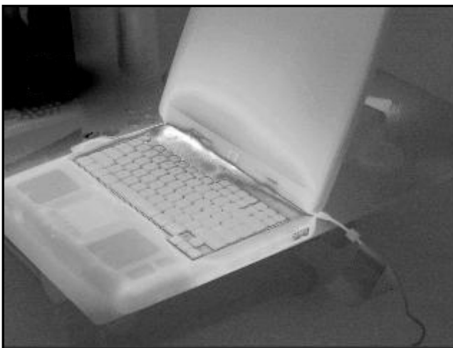
Figure 5 – An image of a normally operating electrical device, in this case a laptop computer, as viewed by a thermal imaging camera. This illustrates how even normally functioning equipment emits heat energy that is observed by a thermal imaging camera. Note the warmer areas are represented by whiter shades indicating warmer temperatures. Cooler areas are represented by darker shades.
