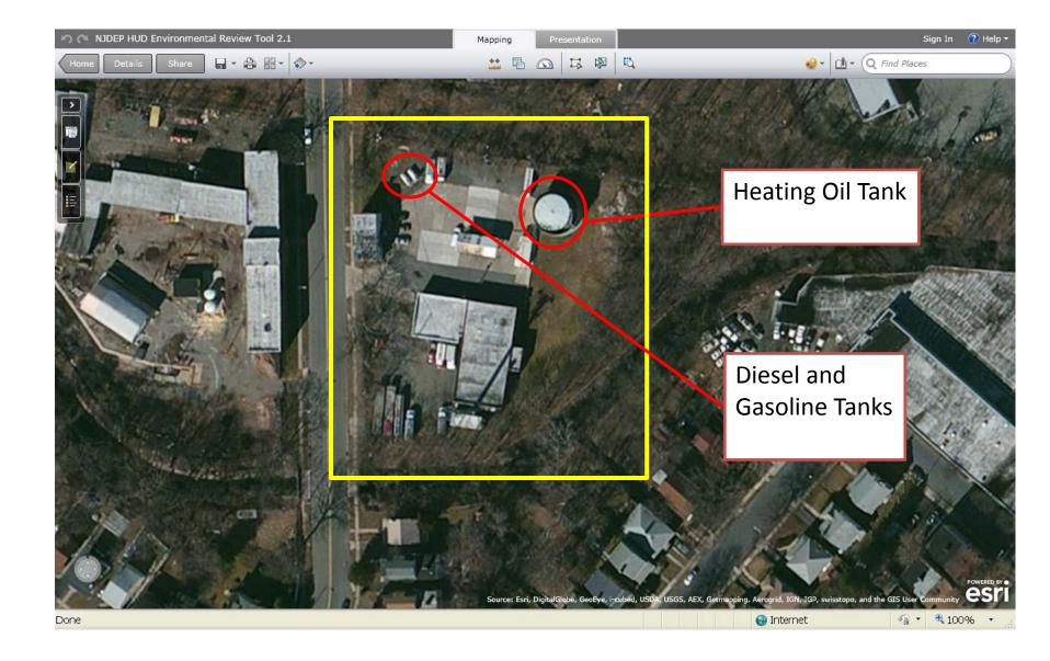
• 250,000 gallon diked Heating Oil tank Diameter is 42 feet.
