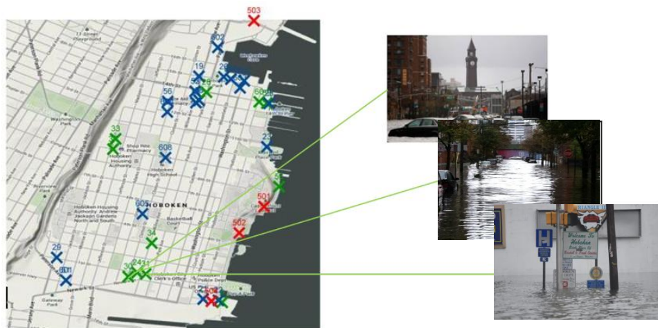
Figure 3-3: Crowdsourcing to Validate Flood Modeling. In partnership with the State, Stevens Institute of Technology is exploring innovative techniques to gather data to inform risk analysis. This photograph is one of many captured both during and following Superstorm Sandy through crowdsourcing. Geo- and time-stamped photos, like this one, allow the State to validate model projections against documented data points, further refining the accuracy of flood modeling to identify areas of increased flood vulnerability.
