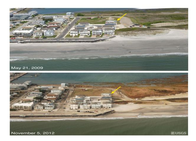
Figure 28 - Storm waves and surge eroded the beach and exposed the seawall during Superstorm Sandy. Overwash of the seawall is indicated by sand deposited on the street. Low dunes on the eastern flank of the seawall were eroded. The yellow arrow in each image points to the same feature.
