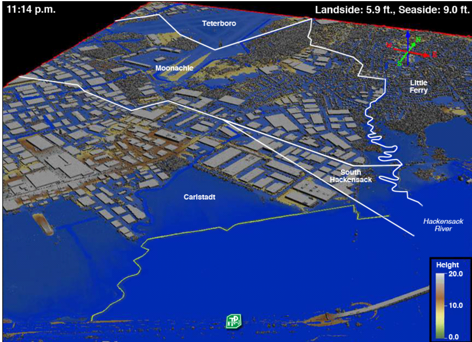
Figure 8: Borough of Moonachie - Surface Water Levels from Sandy, 11:14pm
