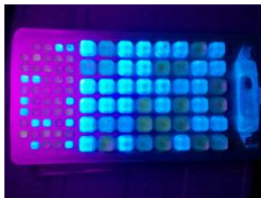
Figure 6: Fluorescent Quanti-Tray/2000 being viewed under a black light.
