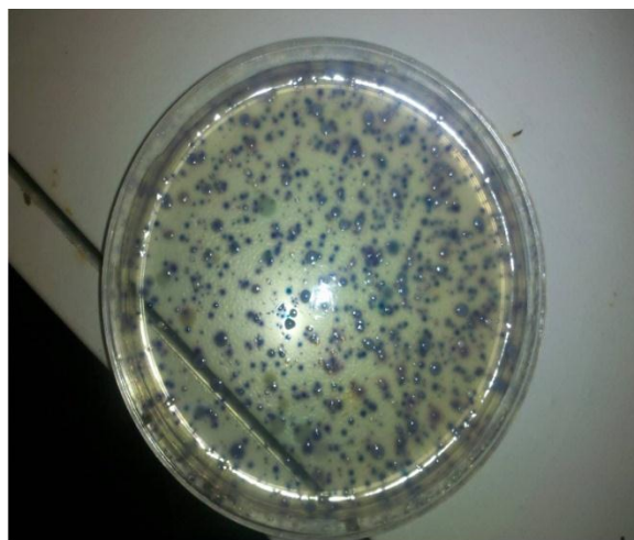
Figure 24: Coliscan petri dish after culturing. The plate represents 41,900 CFUs/100mL from L1S2i.
