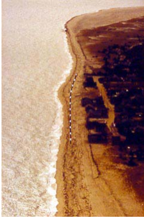
Figure 67. STABEACH ® dewatering system in Cod Fish Park, Nantucket. Dashed line indicates the location of the buried dewatering pipe. Note the bulge in the shoreline generated by the deposition of sediment in the swash zone over the pipe (Photograph courtesy of Coastal Stabilization, Inc.).
