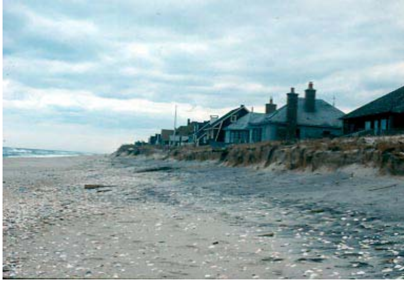
Figure 17b. Similar view of the dune field in Mantoloking, New Jersey after the March 1984 northeaster. Despite horizontal erosion of up to forty feet (40 feet) back into the dune, as well as vertical beach erosion, there were few breaches in this dune field throughout the municipality (Photo courtesy of Dr. Susan D. Halsey).
