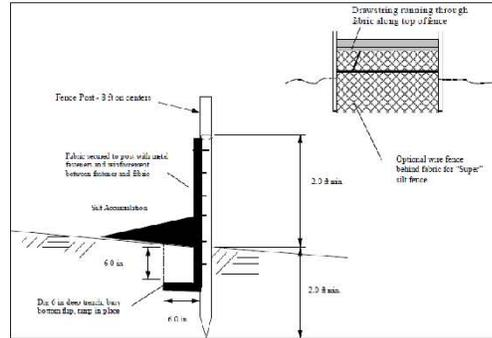
**Typical Silt Fence Detail**
