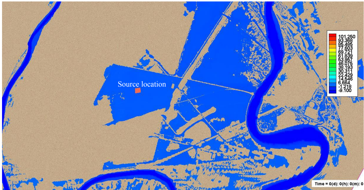
Fig. 5. The contaminant source location in the numerical mesh.
