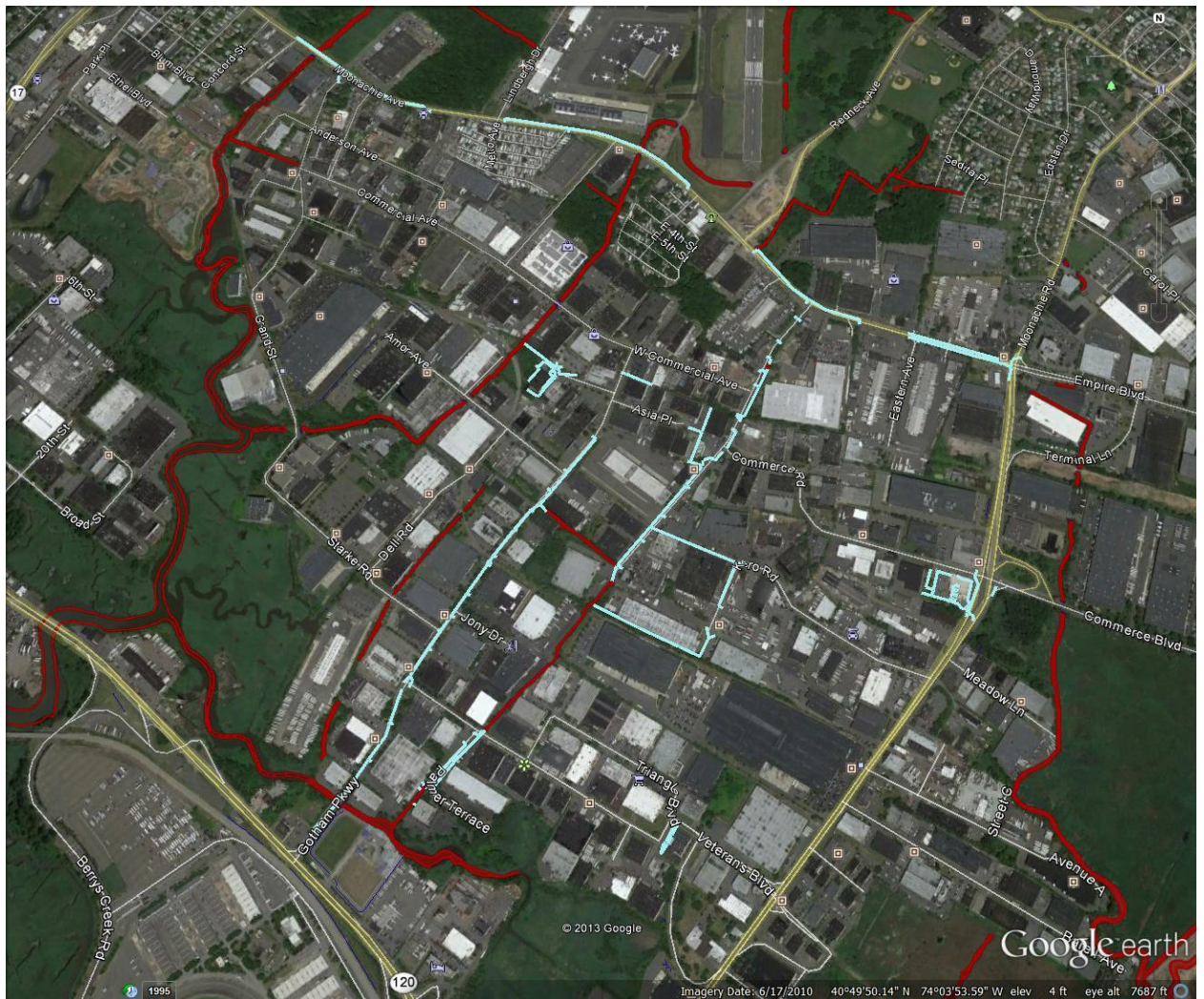
Figure 14: Existing drainage system details for Moonachie, (red-open trenches, blue-gravity mains)
