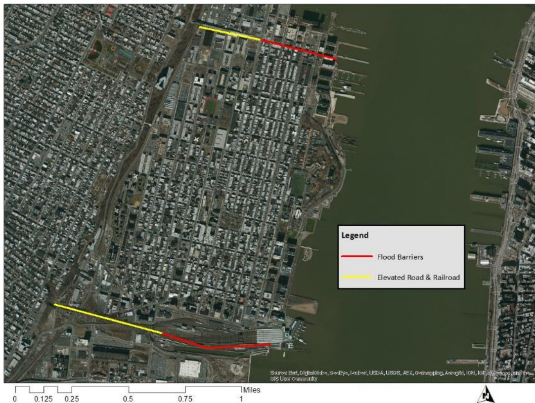
Figure 20: Flood Mitigation Measures Map, Hoboken, NJ.
