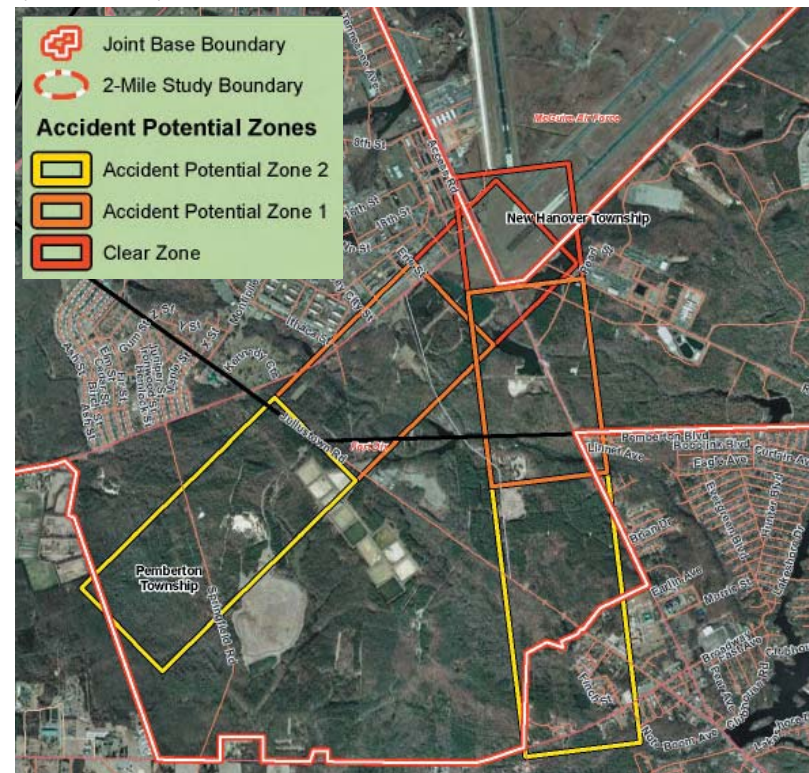
Figure 6.11 Accident Potential Zones for McGuire Runways 06/24 and 18/36 (Southern End)
