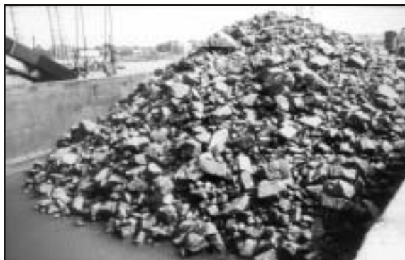
A scow loaded with dredge rock.
