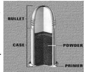
There are two different types of cartridges, they are centerfire and rimfire. Center and rimfire cartridges look similar. The big difference between the two is the location of the primer.
