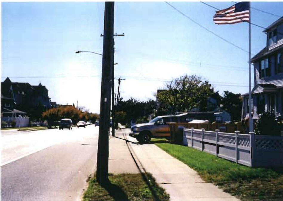
Photo 18: NJ Route 35 in vicinity of Karge Street facing south in Bay Head Borough. This photo shows a cobrahead light affixed to a utility pole and another type of plastic fencing used in the corridor. This fencing is not similar in materials or style to the fencing that lined NJ Route 35 historically and is not a recommended option for use along the corridor.
