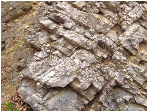
Figure 12. Highly jointed Allentown Dolomite in Kittatinny Valley near Newton. Bedding dips to the left whereas closely-spaced joints dip in the opposite direction. Joints typically exhibit preferred orientations and many are orthogonal to bedding. Joints, fractures, and faults formed during the Taconic and Alleghenian Orogenies when the Lower Paleozoic Formations were tectonically compressed.
