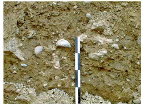
Figure 16. Compact sandy-silty till, Kittatinny Valley. Chiefly derived from local dolomite, shale, and sandstone. Divisions on scale equal one foot.
