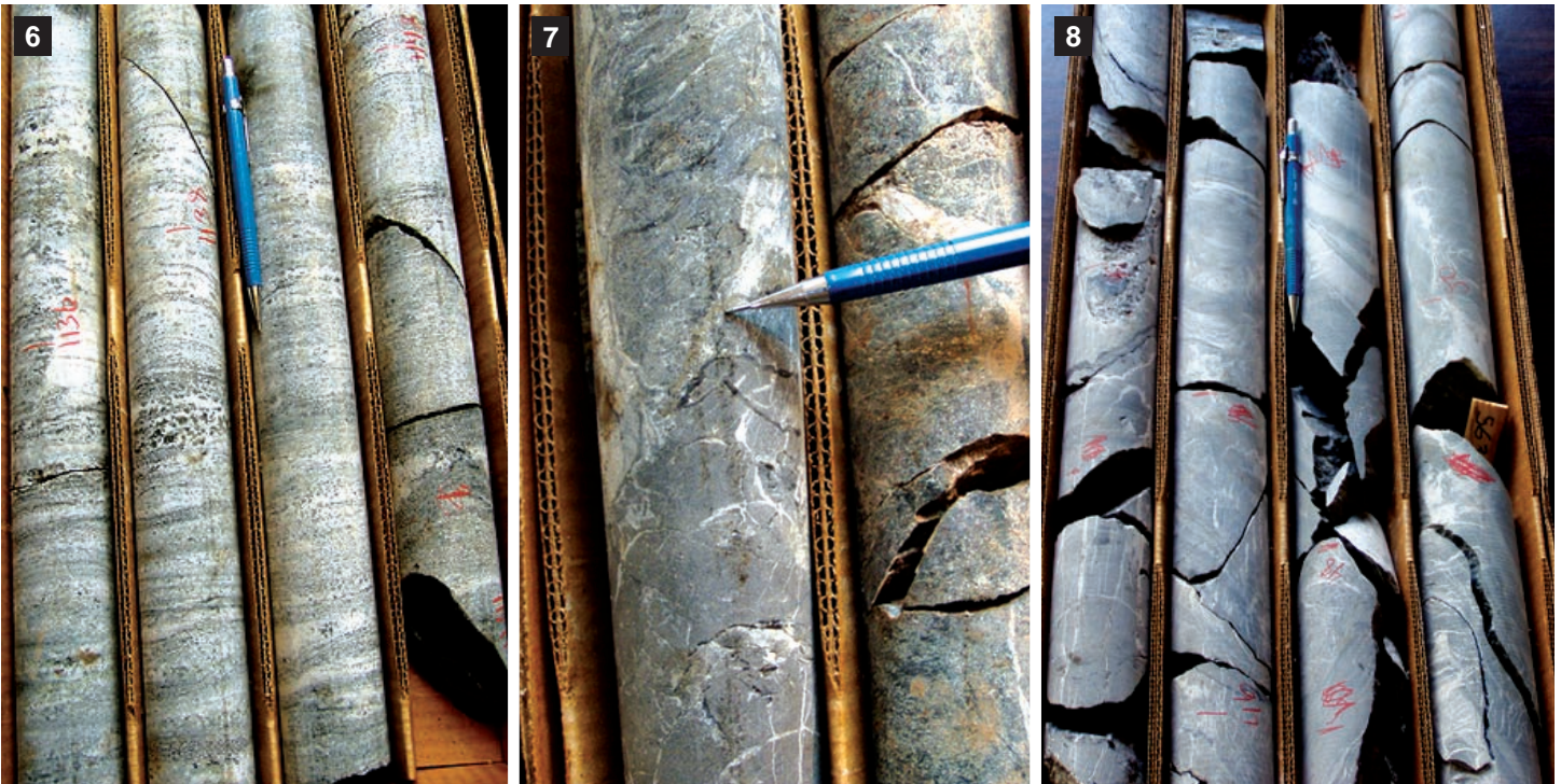
Figure 6, above left. Drill core of strongly-banded Precambrian gneiss penetrated in hole DR1. Figure 7, above center. Close-up of thrust fault between Precambrian gneiss (top) and Paleozoic dolomite (bottom) in drill core from hole DR2. Fault plane in the core dips at an angle of about 60°, but the dip becomes much gentler to the east of the corehole. Pencil tip points to the fault contact. Figure 8, above right. Drill core of Paleozoic dolomite encountered beneath the thrust fault in hole DR2. Photos by R.A. Volkert
