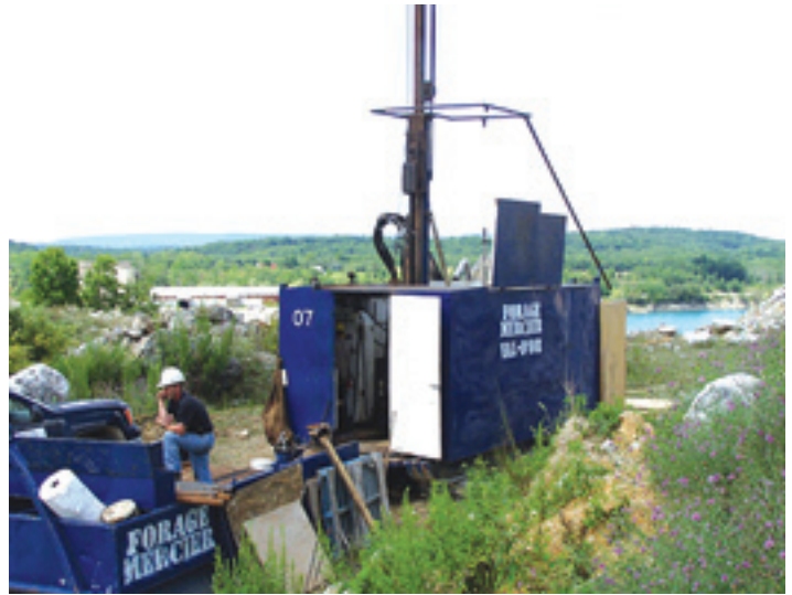
Figure 3. Forage Mercier drill rig and the principal driller at corehole DR1, at the south corner of the quarry. Photo by R.A. Volkert
