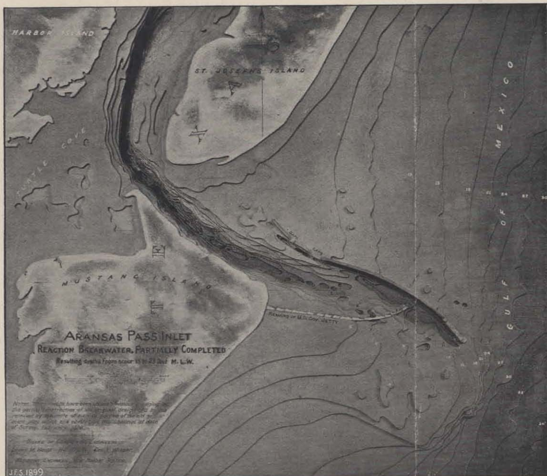
Aransas Pass, Texas, showing improvements up to 1901, and the consequent deepening of the channel.
