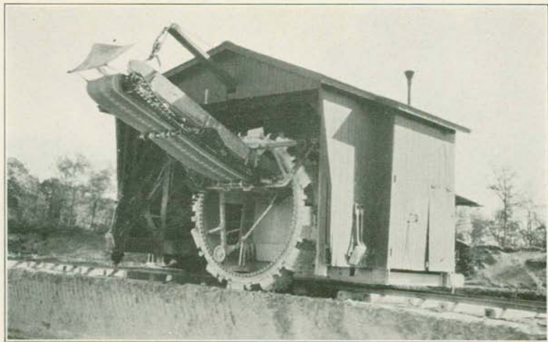
(a) Clay-digging machine used by the Crossman Company in its large pit near Parlin.
