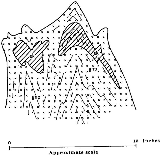
**FIGURE 2**—Sketch showing small skarn pods in crests of tight folds in pyroxene-feldspar gneiss, near Tar Hill mines. Note extreme thinning or absence of skarn on limbs of folds. sk, skarn; gnp, pyroxene gneiss
