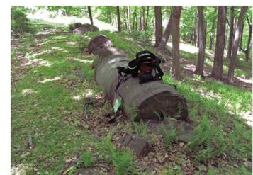
36 inch (91 cm) diameter calyx core along the Rock Cores Trail, Worthington State Forest, New Jersey. The core was drilled in the Bloomsburg Red Beds during the geologic investigation of the Tocks Island dam site during the 1950s. Geologists were suspended in steel cages down the bore shafts in order to log the bore holes. Photo by R. Witte.
