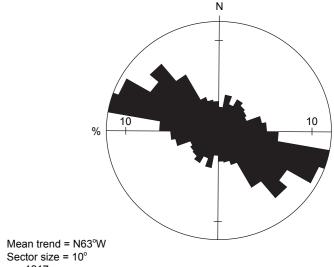
n = 1217 Figure 2. Rose diagram of 1,217 joint orientations in Mesoproterozoic rocks.
