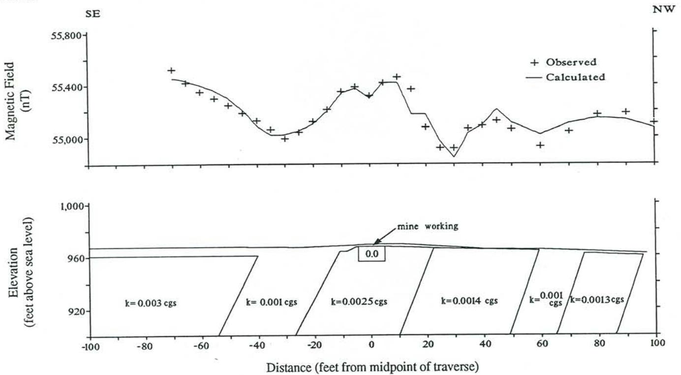
Figure 3. Magnetic profiles for lines 1 and 2 showing observed magnetic data with calculated data from models.
