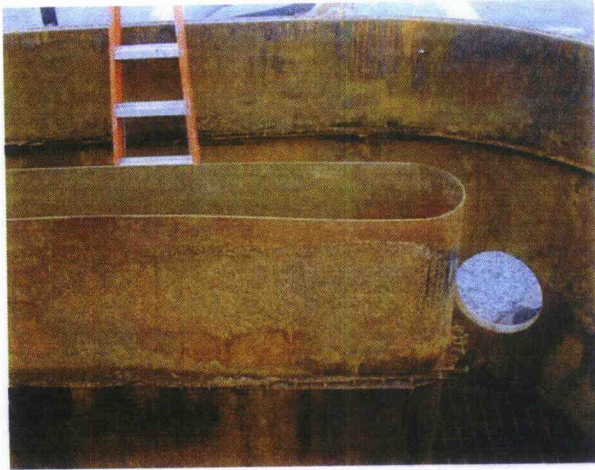
Figure A-15. Inside of Activated Carbon Bed and Central Flue Gas Chimney (The lower grating without screen is also shown)
