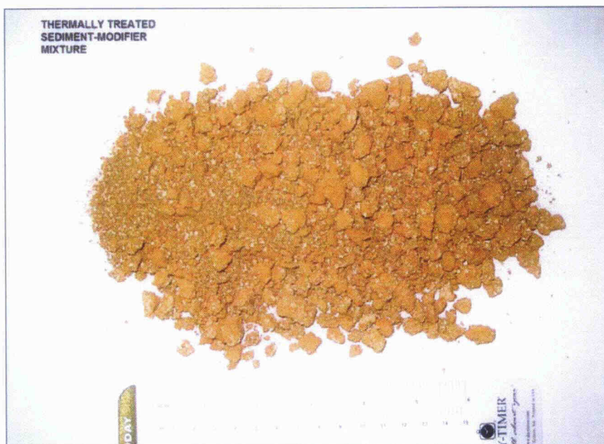
Figure 4. EcoAggMat Produced in Laboratory-Scale Furnace
