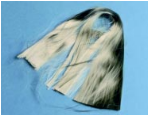
Figure 7-12. Photograph of fiberglass fabricated from the glassy material produced with the Westinghouse plasma torch. This is a possible beneficial use for the treated dredged material.
