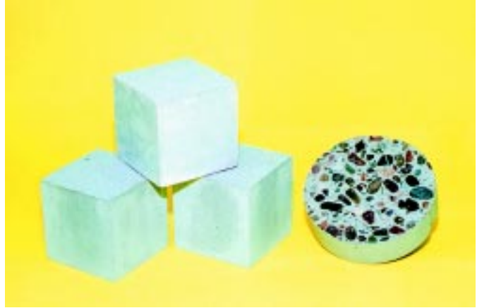
Figure 7-9. Cement blocks and paving material produced following high temperature treatment in the pilot-scale demonstration performed by the Institute of Gas Technology.
