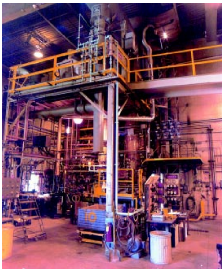
Figure 7-10. Photograph of the Westinghouse Science and Technology Research Center 2 megawatt plasma torch facility.
