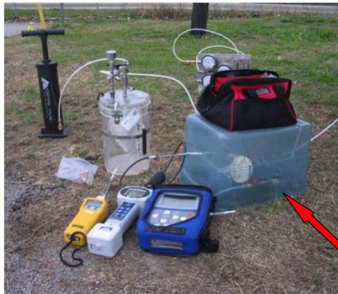
Figure 3-1 Schematic diagram of sampling train using leak detection and photograph of helium shroud with Summa Canister (courtesy Geosyntec Consultants)
