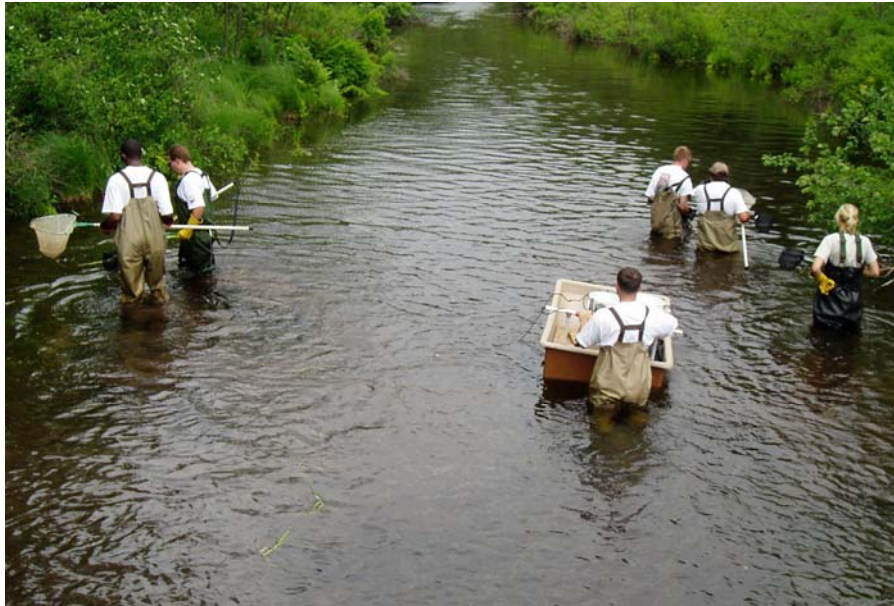
Figure 2. A typical fish sampling operation using the electrofishing barge.
