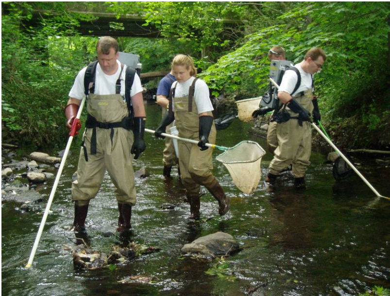
Figure 2. A typical fish sampling operation using the backpack electrofishing.
