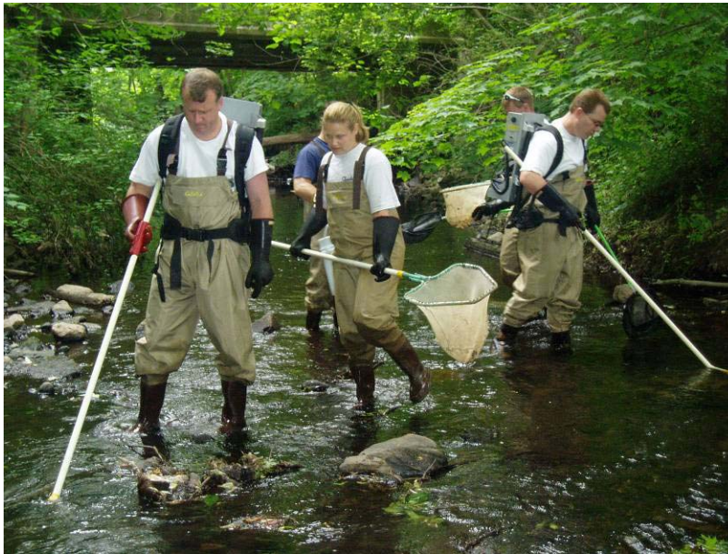
Figure 2. A typical fish sampling operation using the backpack electrofishing.
