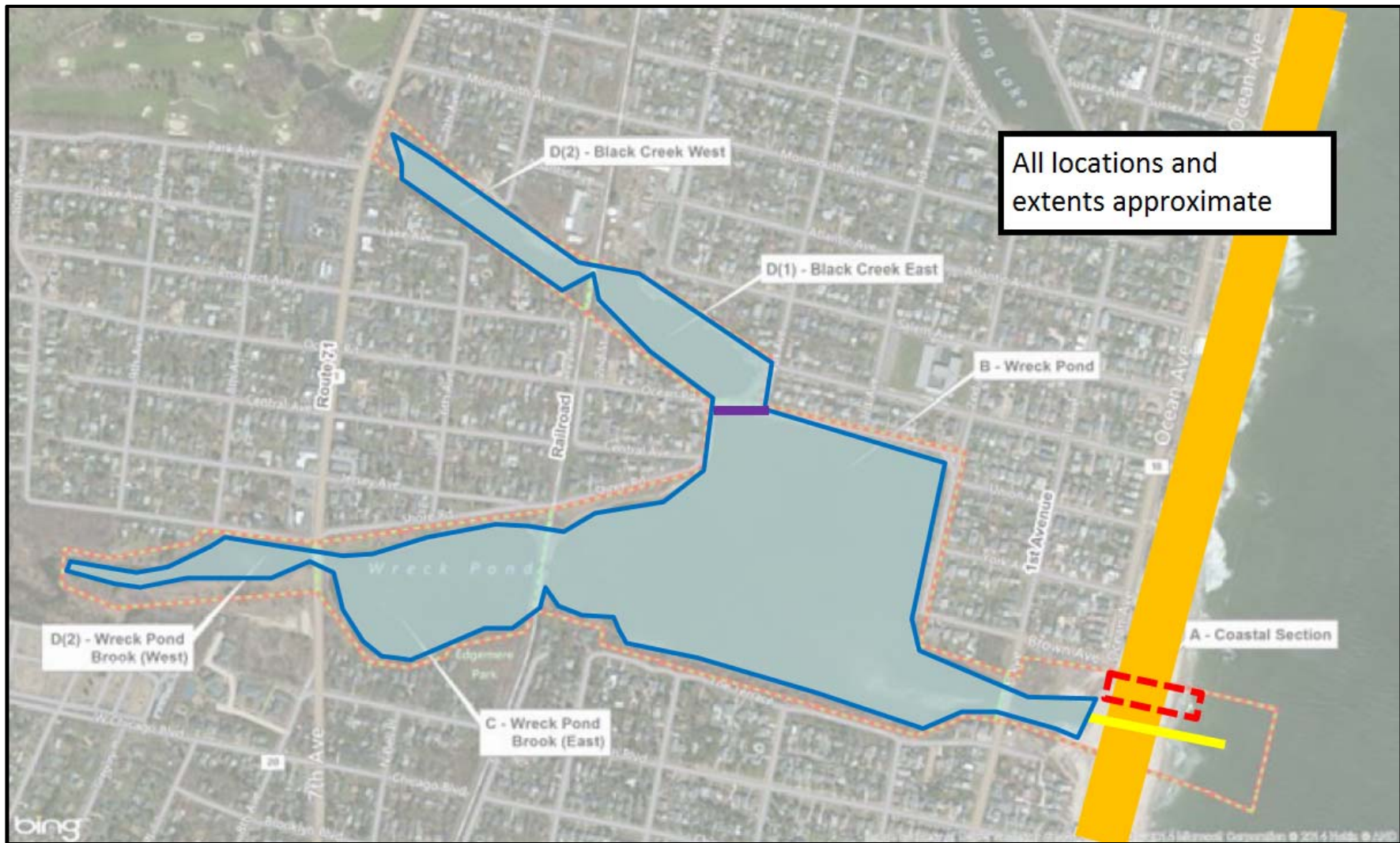
Figure 16: Existing water resource projects. The extent of Wreck Pond is shown in blue. USACE beach nourishment project (orange), outfall pipe (yellow), Black Creek weir (purple), and temporary emergency spillway (red). Pond dredging in various locations in the pond. Stormwater infrastructure at various locations.
