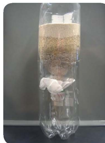
water filter set-up
