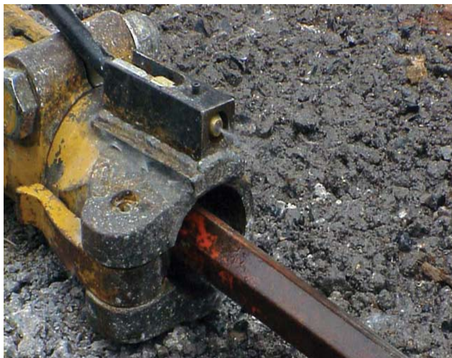
Figure 1. The water spray attachment, showing the method used to attach the nozzle to the tool.
