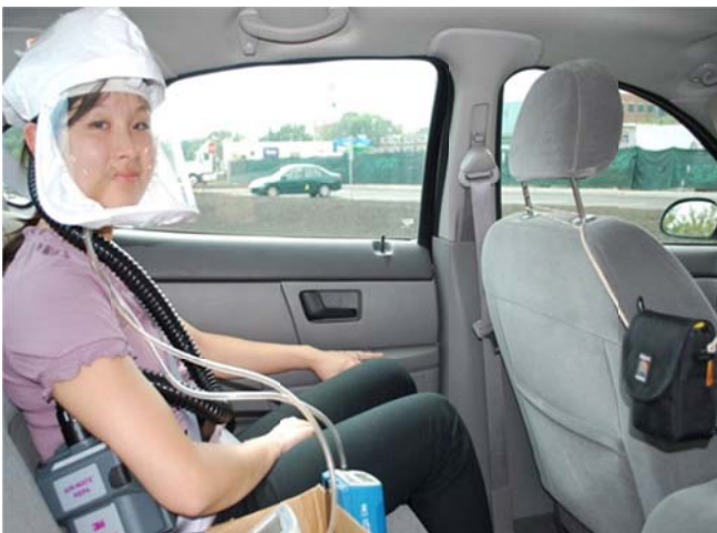
One of the investigators demonstrates how the comfortable, light-weight air purifying respirator was worn by the participants in the study.
