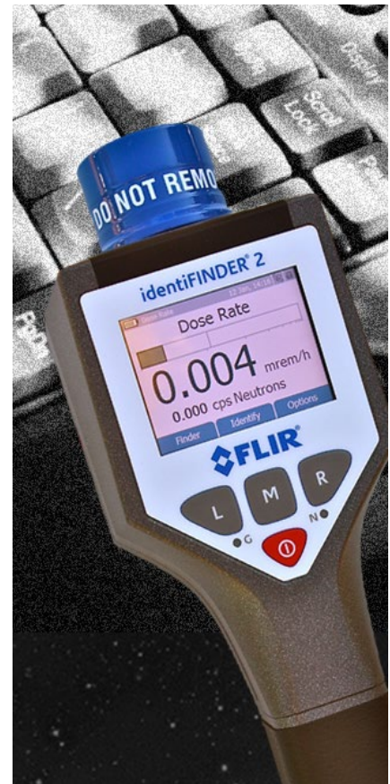
Radiation Isotope Identifier Device—CTOS/NNSA
