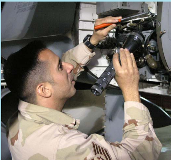
Crew Chief Tech. Sgt. Frank Spano checks the forward avionics bay on an F-16 during the aircraft's phase inspection.
