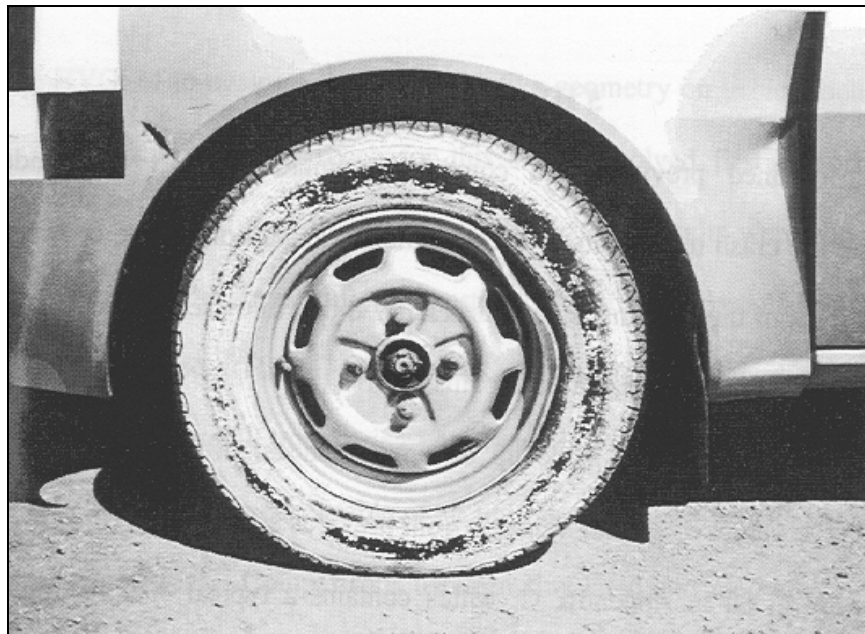
Figure 17. Wheel Damage after Full Scale Crash Test (photo taken from Holloway, J.C., Sicking, D.L., Rosson, B.T., 1994)
