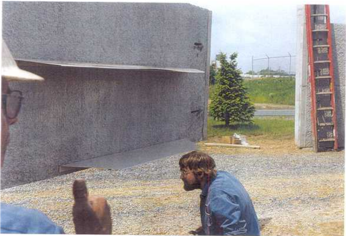
Fig. 18 6 ft. fin above 4 ft. fin shows some edge waviness.
