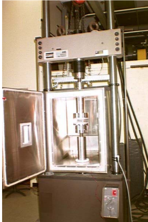
Figure 2: Photograph showing the setup of the MTS machine with an environmental control chamber.
