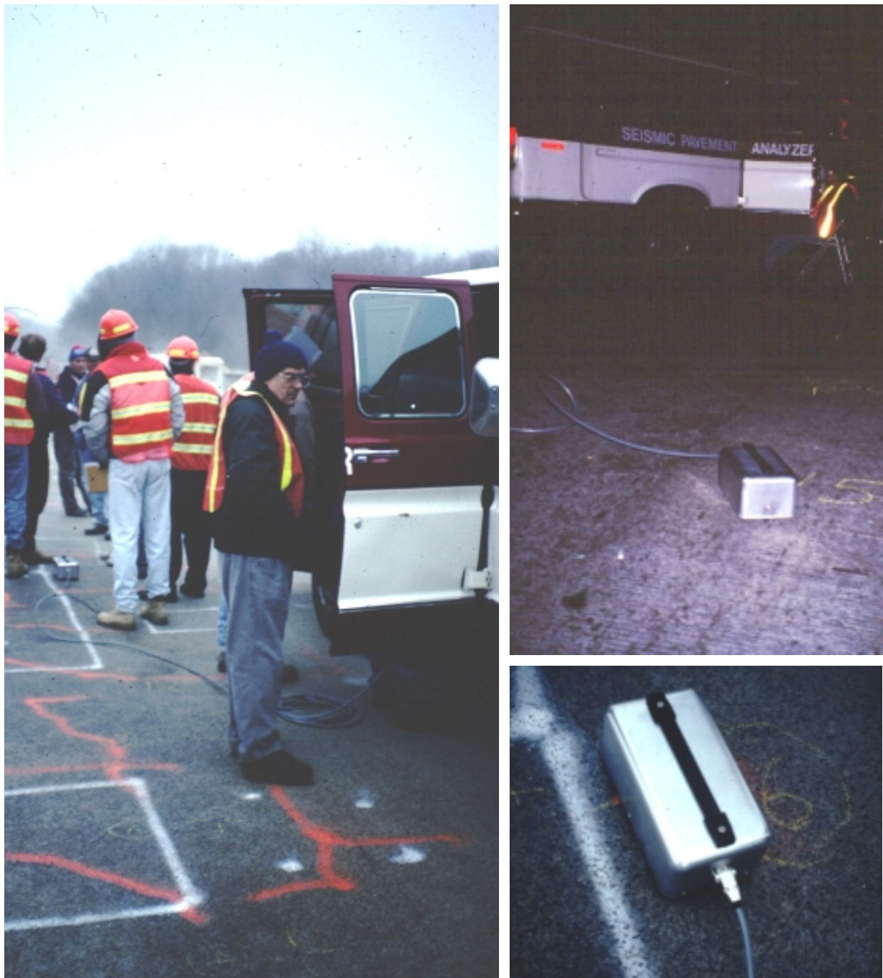
Figure 4.2. Evaluation of bridge decks by PSPA.
