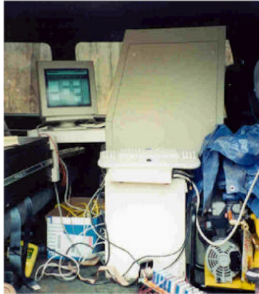
Figure 13 The data acquisition unit. The monitor shows the graphical representation of the ratchet loading.
