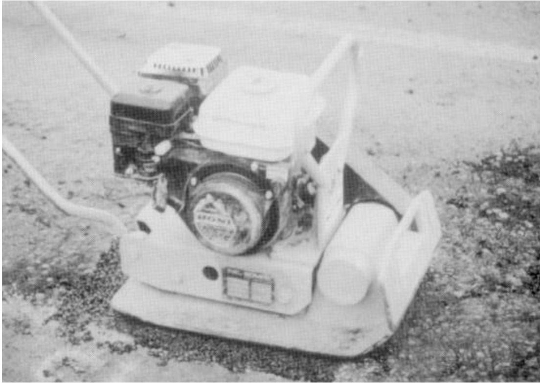
Figure 9. Semi-permanent Method of Pothole Repair: Compaction Using a Mobile Vibratory Plate Compactor (5)
