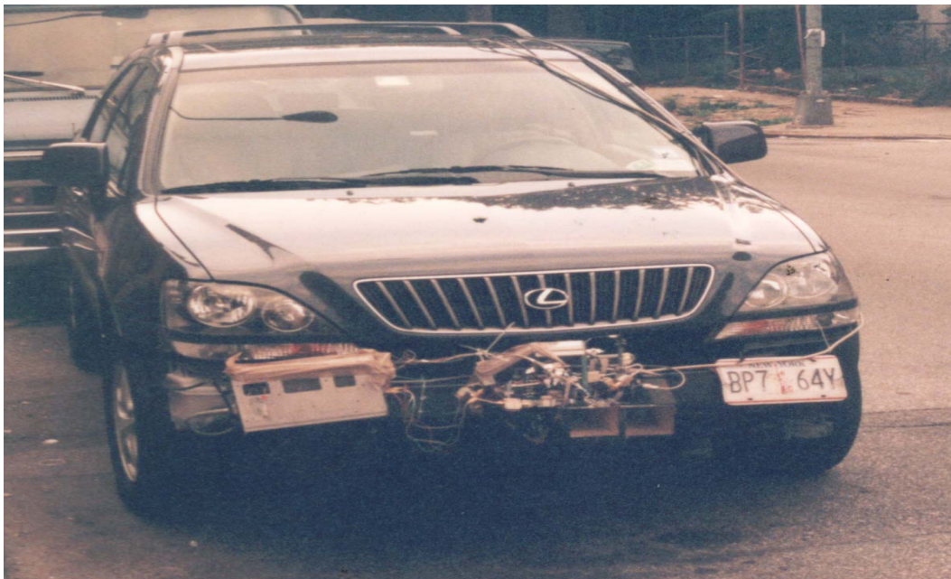
Figure 2. Field tests were performed using a radar, constructed with waveguide components installed on the front bumper of the vehicle.
