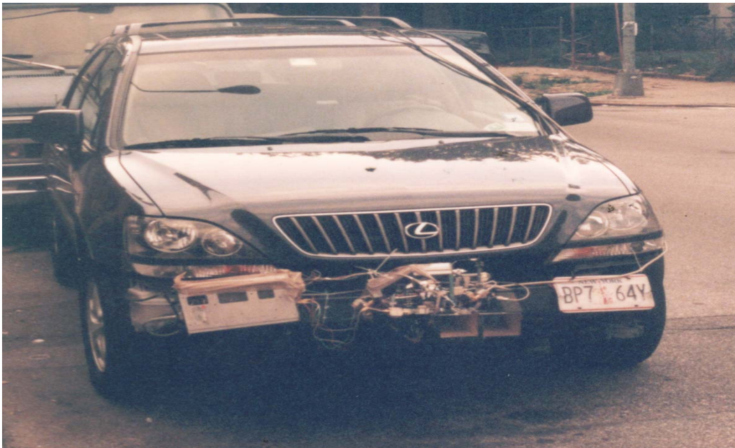
Figure 4. Field tests were performed using a radar, constructed with waveguide components installed on the front bumper of the vehicle.
