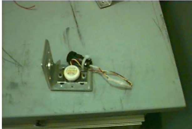
Figure 7-9. Accelerometer mounted to testing plate
