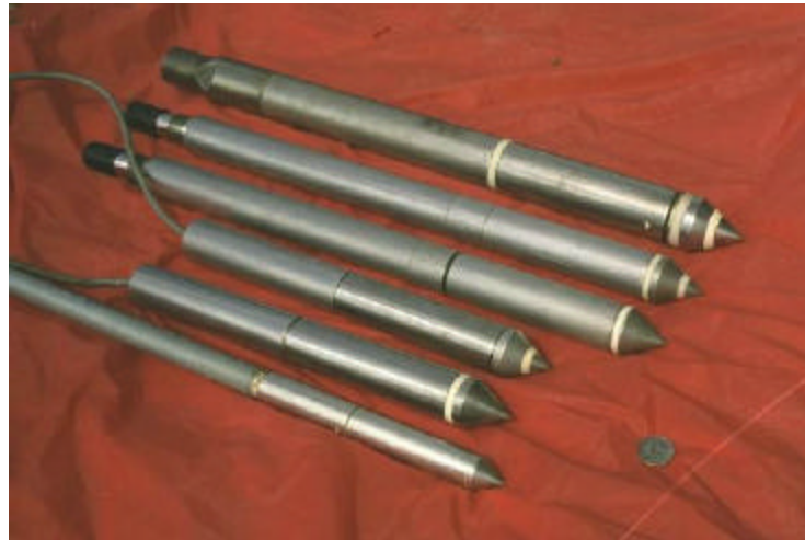
Figure 1 – Different Cone Penetrometers Used for Site Investigation
