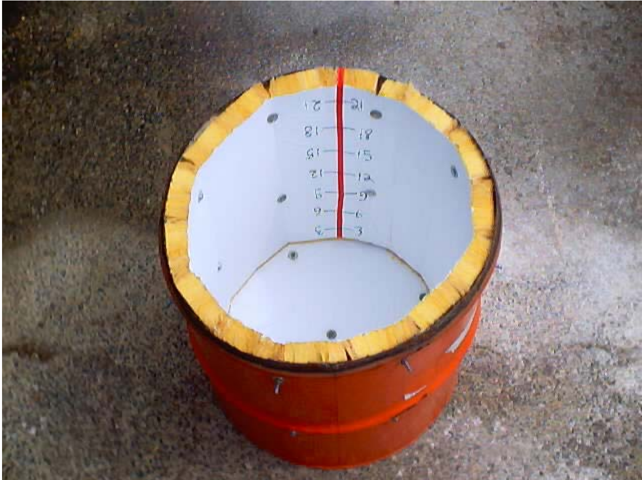
Figure 4 – Small “Soil Bin” Used for Laboratory Evaluation of the HSG
