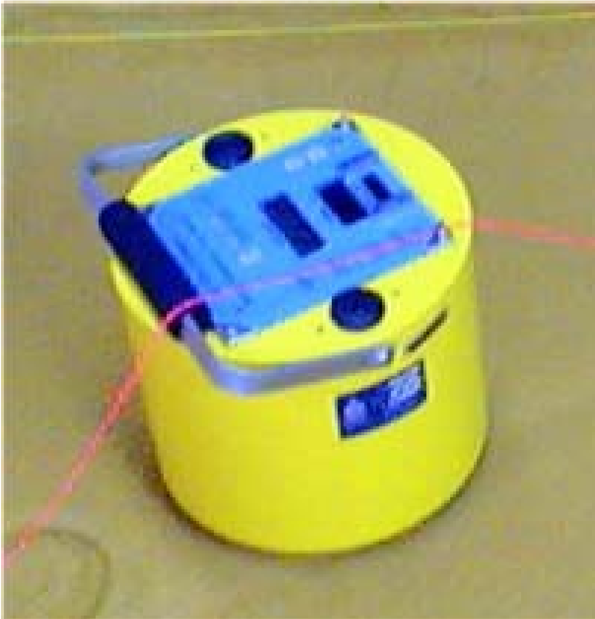
Figure 1 – The Humboldt Stiffness Gauge
