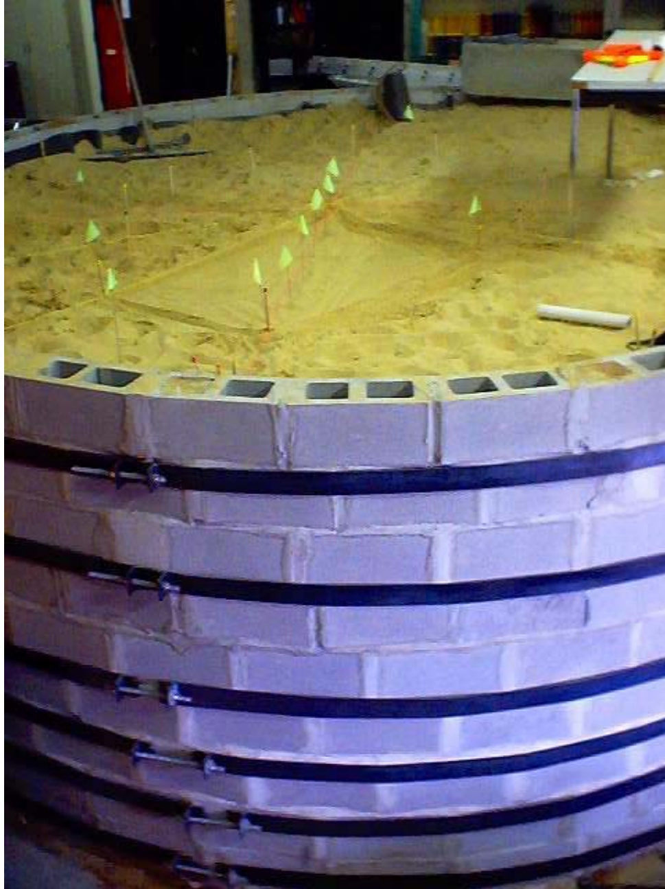
Figure 12 – Large Test Bin Used for HSG Evaluation
