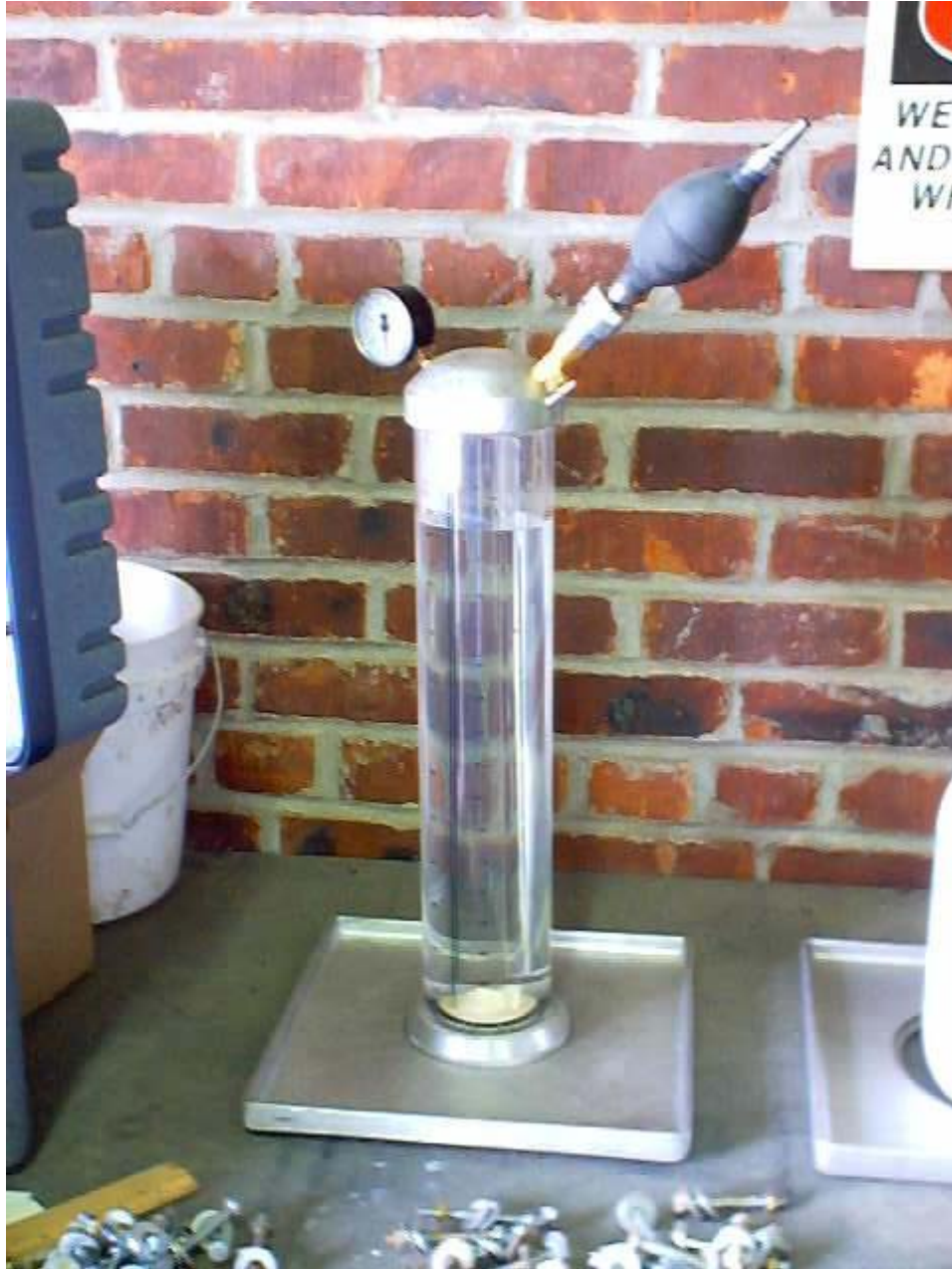
Figure 11 – Rubber Balloon Density Test Apparatus
