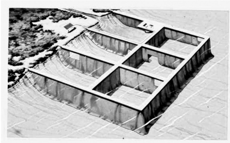
Figure 5: Flow balancing system schematic (Courtesy Fresh Creek Technologies)
