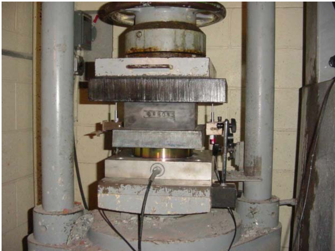
Figure 2A. Square bearing being tested in pure compression.
