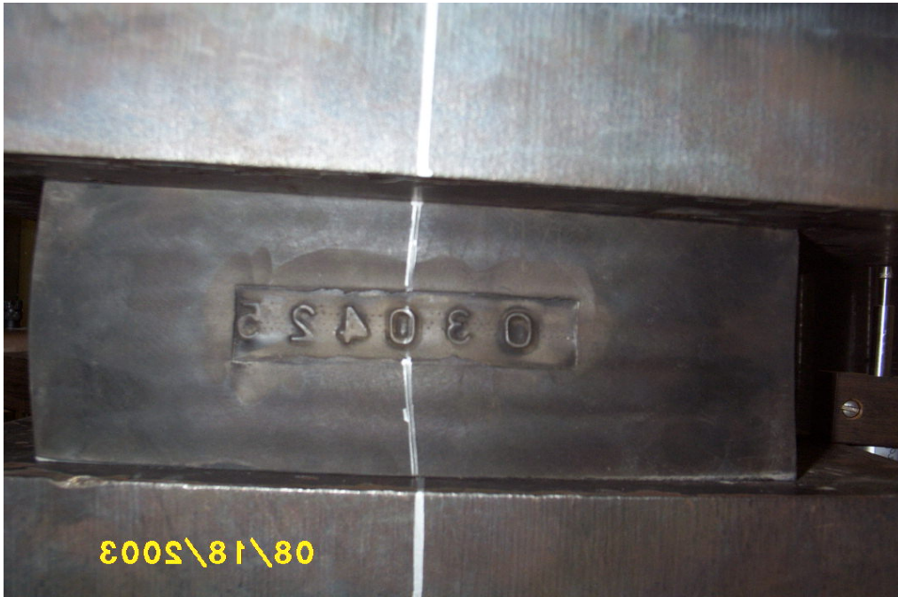
Figure 3A. Square elastomeric bearing during compression and rotation tests.
